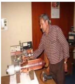
Fig. 9 Leak testing of GCTM
