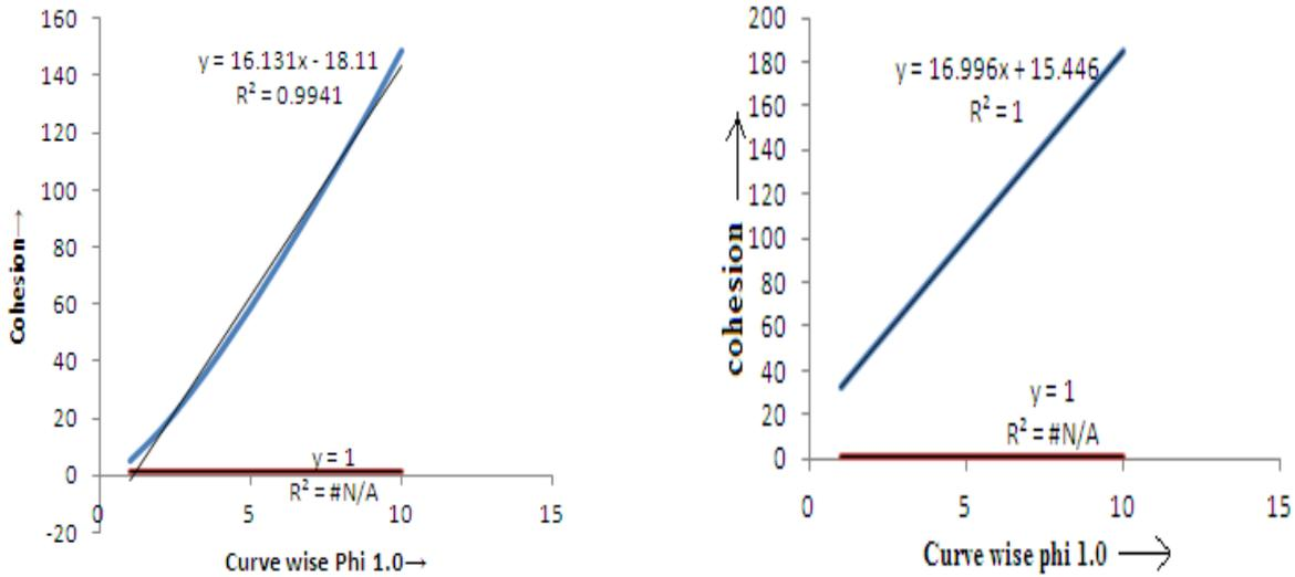
Fig. 6 Relationship between cohesion calculated for minimum value of phi 1.0 for tunnel-1 and tunnel- 2
