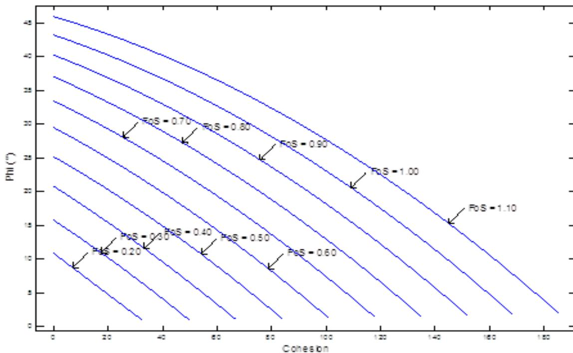
Fig.3 Multiple back analysis-bishop simplified method of analysis of Khokhariyanal tunnel-2 SSE cut face
