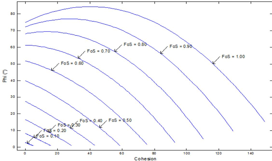
Fig. 2 Multiple back analysis-bishop simplified method of analysis of Ukhaliyat tunnel-1 SSW cut face
