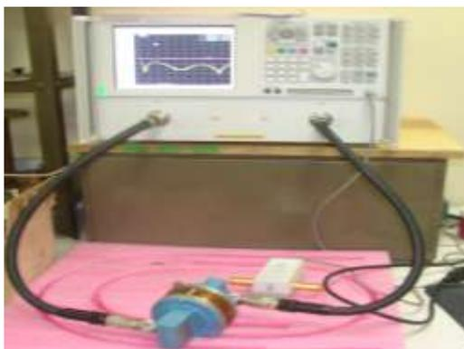
Fig. 9 C band window in test bench
