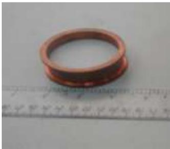
Fig. 7 Fabricated C band window
