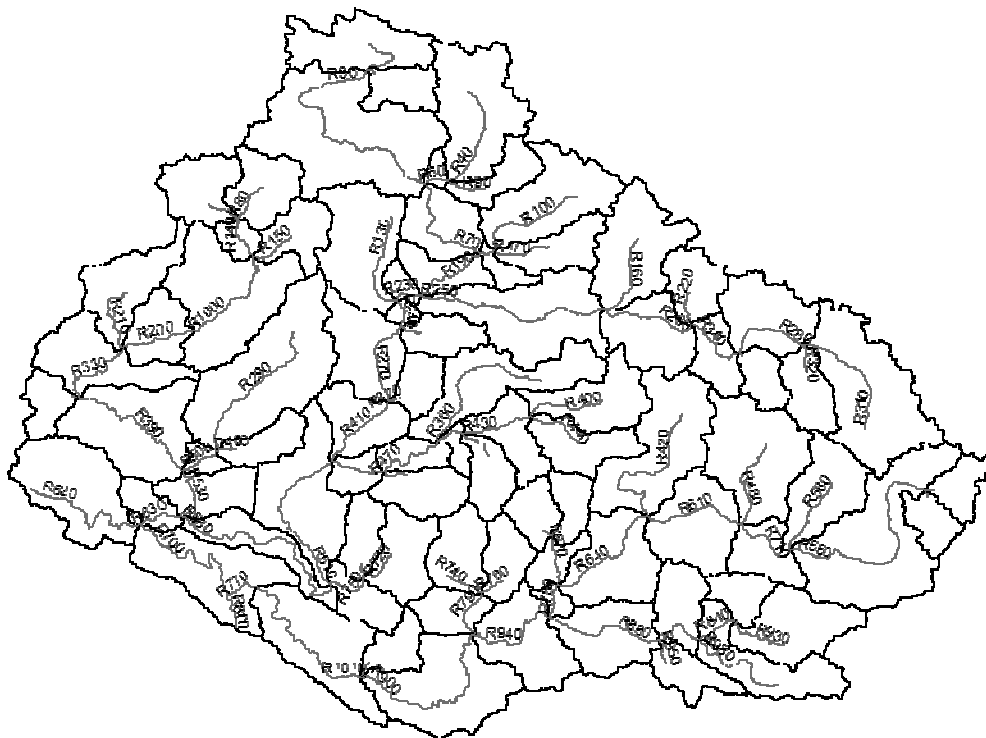
Fig. 6 River Network Extracted from HEC Geo HMS with 85 Numbers of Sub-Basins
