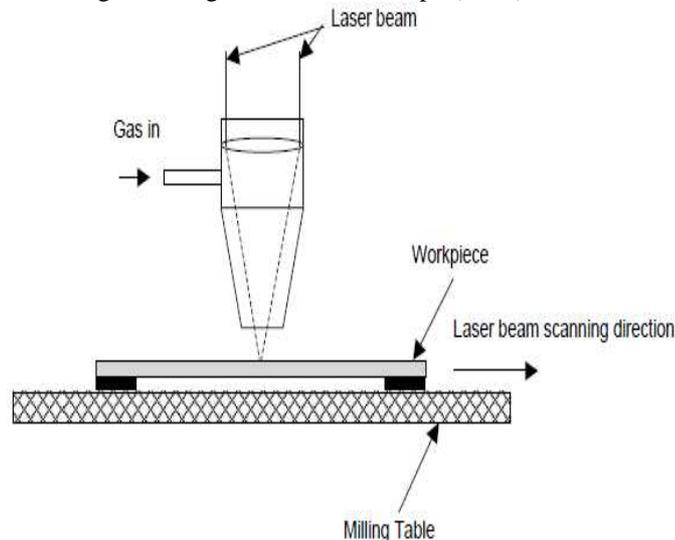
Fig. 8 Schematic view of the experimental set-up (Yilbas [13])
