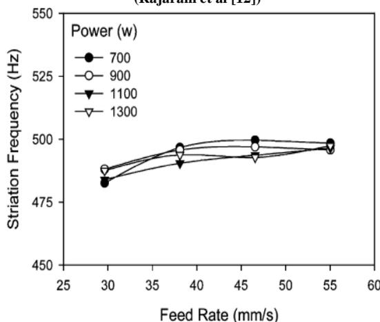
Fig. 6 Variation of striation frequency with power and feed rate (Rajaram et al [12])
