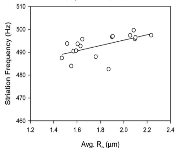
Fig. 7 Correlation between striation frequency and surface roughness (Rajaram et al [12])
