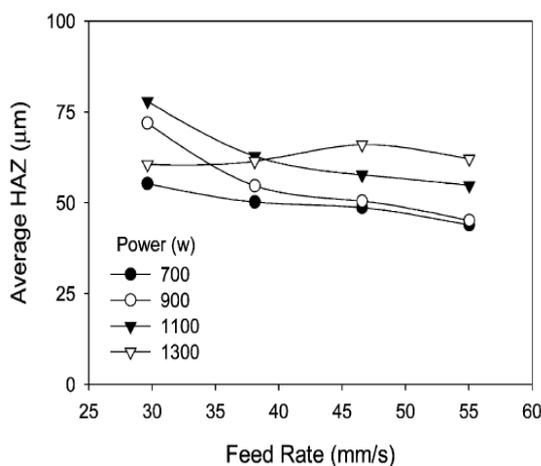
Fig. 4 Variation of HAZ width with power and feed rate (Rajaram et al [12])
