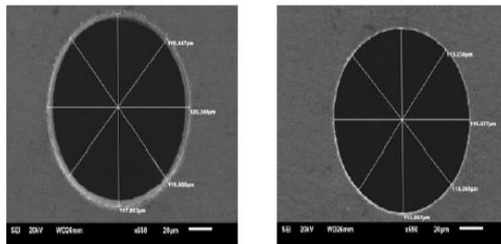
Fig. 10 SEM images of the entry and exit micro-holes produced by micro-EDM (Rasheed (2013), [15])
