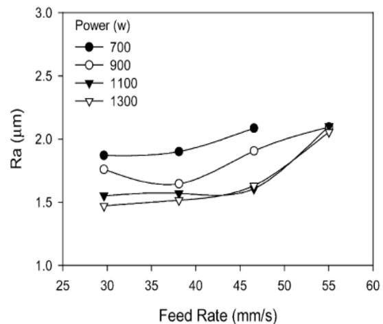
Fig. 5 Variation of surface roughness with power and feed rate (Rajaram et al [12])
