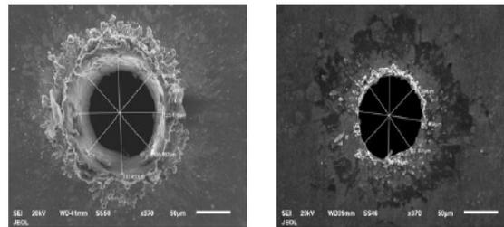
Fig. 9 SEM images of the entry and exit micro-holes produced by LBM (Rasheed (2013), [15])
