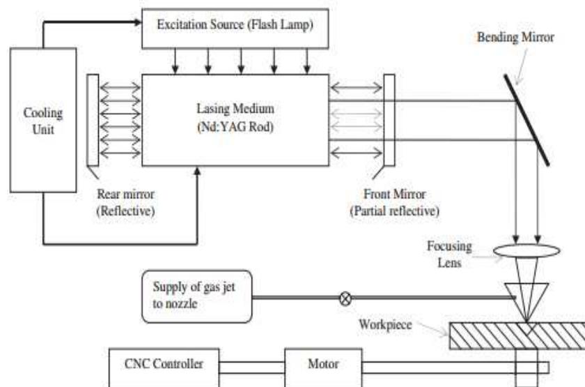
Fig. 1 Schematic Representation of Nd-YAG Laser Beam Machining (Dubey and Yadava [7])
