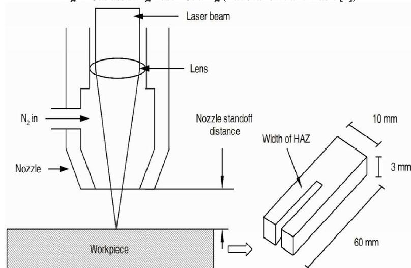
Fig. 3 Nitrogen assisted Laser Cutting Of AISI 3140 Steel (Radovanovic and Madic [4])
