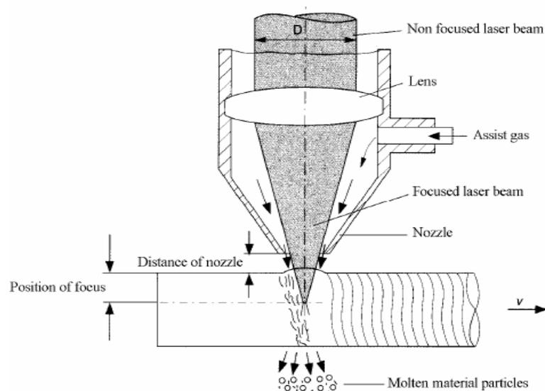
Fig. 2 Gas assisting Laser Cutting (Radovanovic and Dasic [5])
