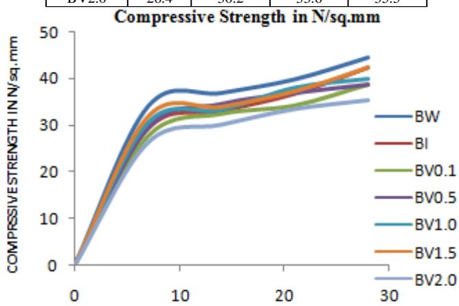
**Fig. 2 Compressive strength vs. Age of curing**
