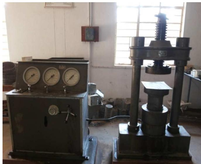
**Fig.1 (d)** Compressive testing machine
