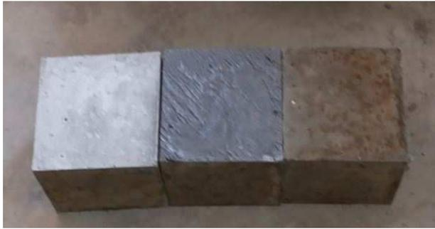
Fig.1 (a) Cubes after demoulding
