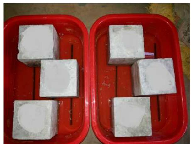
**Fig.1 (f)** Specimens under sorptivity test
