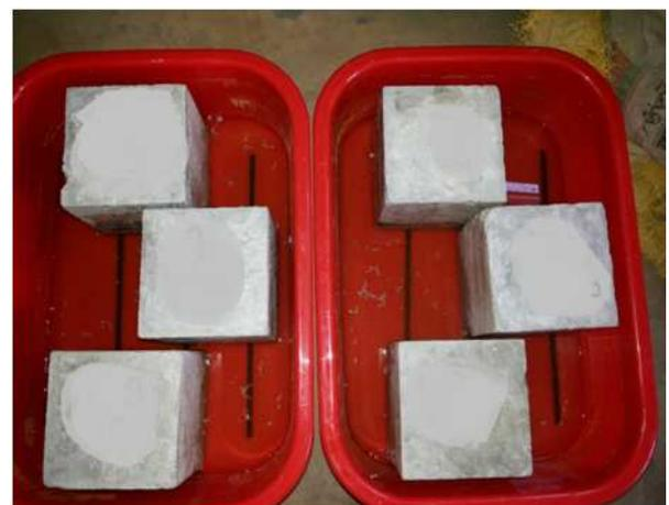
Fig.1 (f) Specimens under sorptivity test
