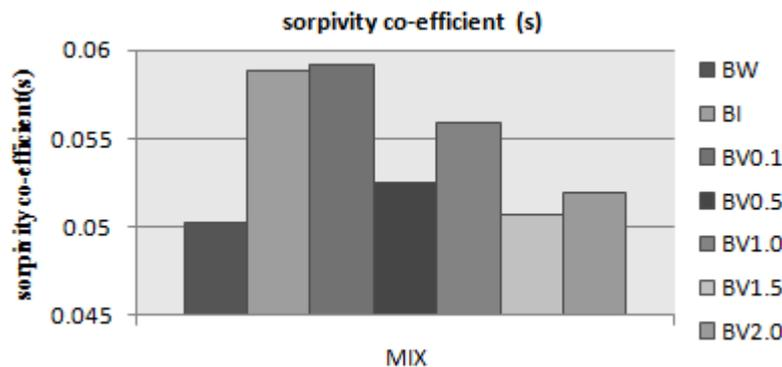
**Fig. 5 Sorptivity co-efficient (s) vs. mix proportions**
