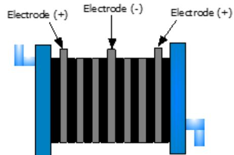
Fig. 7 HHO generator with three electrodes applied
