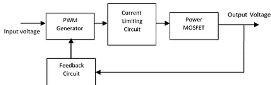
Fig. 12 Block diagram of the Electronic Circuit
