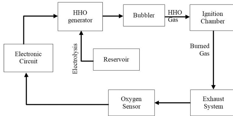
Fig. 13 Block diagram of the Complete System
