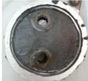
Fig. 9 Corroded Zinc coated iron plate
