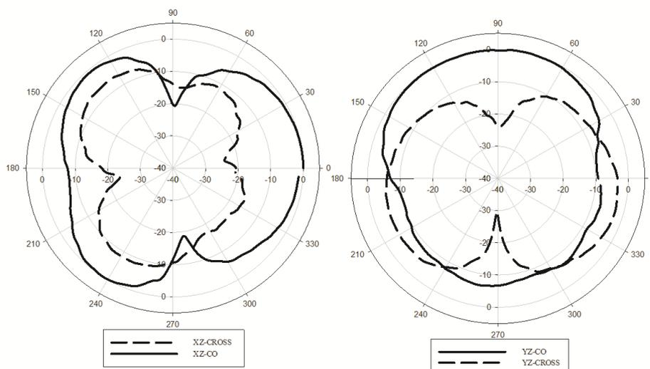
Fig. 12 Radiation Pattern at 5.8GHz
