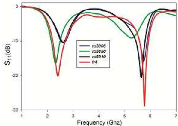
Fig. 10 Reflection Characteristics on different substrates
