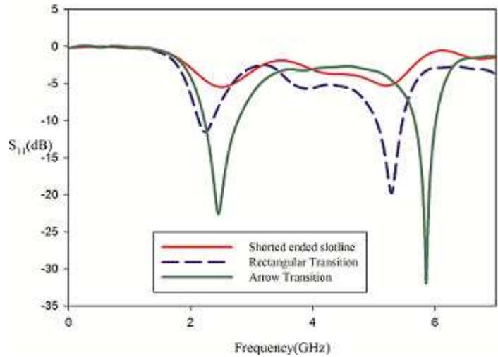
Fig. 2 Reflection Characteristics
