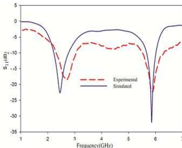
Fig. 3 Reflection characteristics of the fabricated prototype
