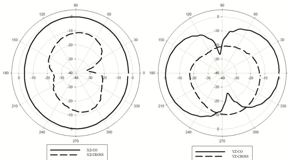
Fig. 11 Radiation pattern at 2.4GHz
