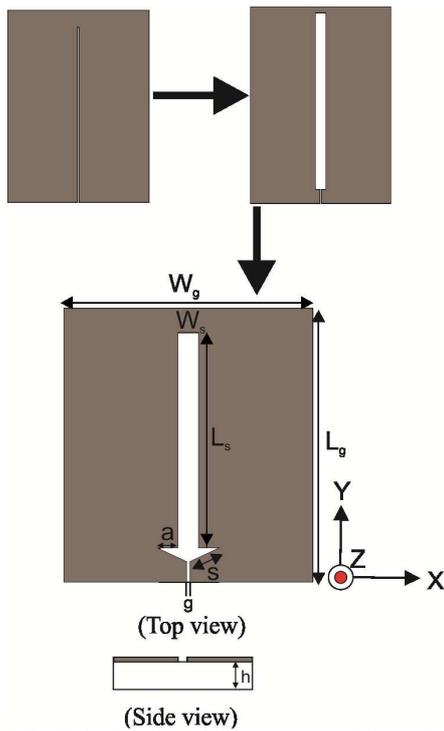
Fig. 1 Optimised design of the antenna and its evolution
