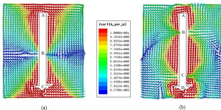
Fig. 9 Surface current distributions (a) 2.4GHz (b) 5.8GHz
