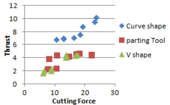
Fig. 11 Effect of Tool Shape on Cutting & Thrust Force
