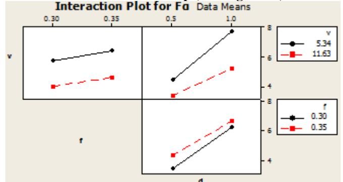
Fig. 9 Interaction Plot for Cutting Force among Speed, Feed and Depth of Cut
