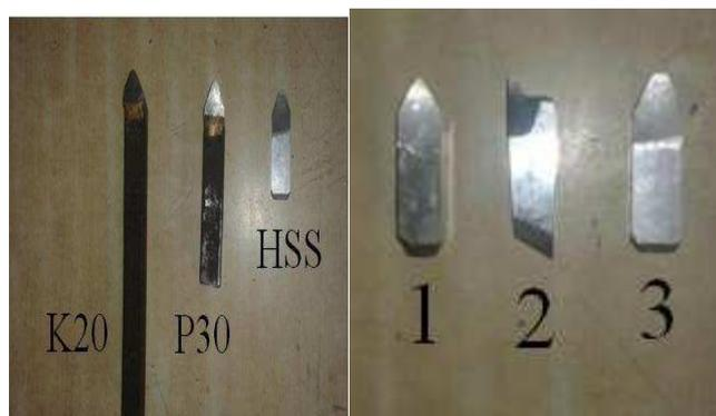
Fig. 5 Different Tool Materials & Shapes
