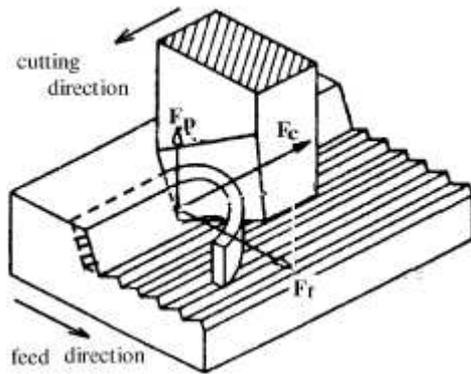
Fig. 3 Mechanism of Shaping Operation [15]
