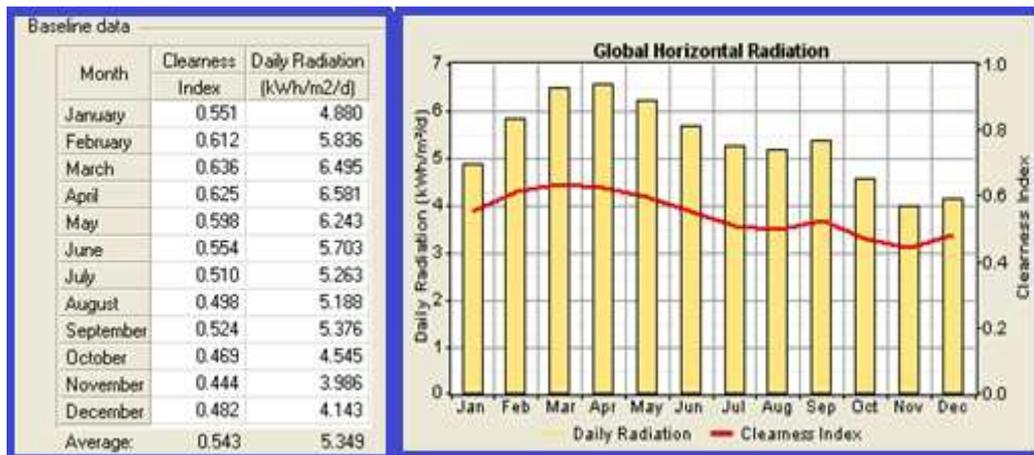
Fig. 4 (a) Solar radiation location input (b) Monthly radiation data (c) Solar resource inputs
