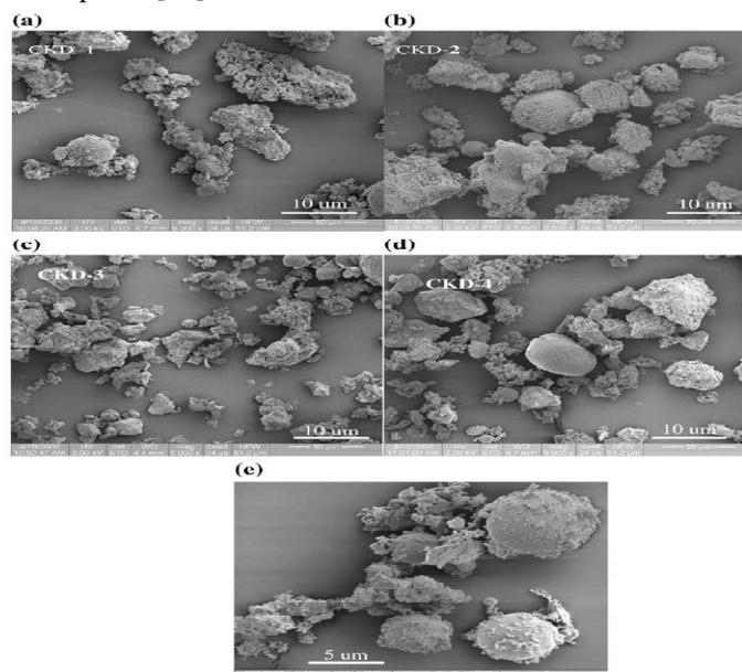
**Fig.1** Scanning electron micrographs of CKD powders: (a) CKD-1, (b) CKD-2, (c) CKD-3, (d) CKD-4, (e) close-up-of the cluster containing both the agglomerated and spherical particles covered with very fine deposits in CKD-1 [Peethamparan *et al* (2008)]
