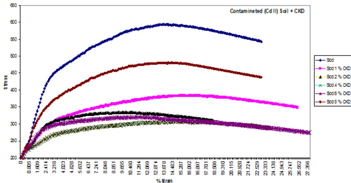
Fig.7 UCS values of Cd contaminated soil and contaminated soil-CKD mixes
