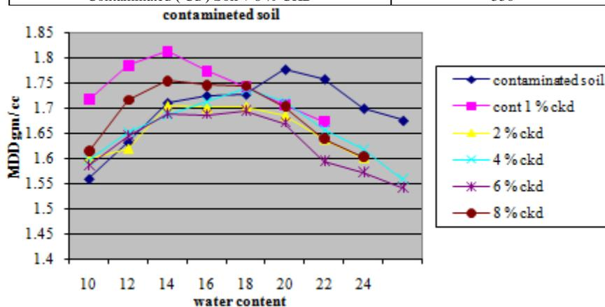
Fig. 6 OMC-MDD curve of Cd contaminated soil and contaminated soil-CKD mixes
