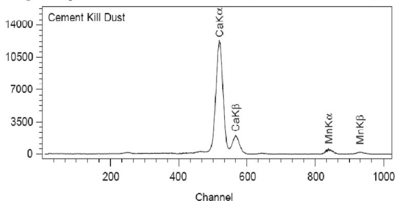
Fig.3 X-ray spectrum obtained for CKD specimen using  $^{55}\text{Fe}$  excitation [Polat et al (2004)]
