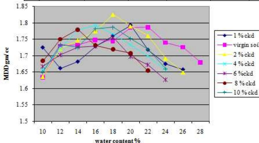
Fig. 4 OMC-MDD curve of virgin soil and virgin soil-CKD mixes
