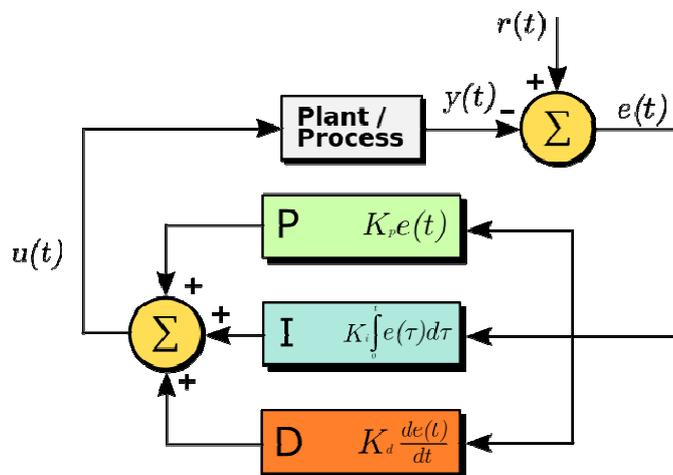
Fig. 12 Block diagram of PID-Controller
