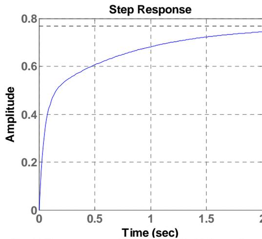
Fig. 11 Time response of DC motor with PI-Controller
