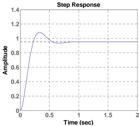
Fig. 7 Time response of DC motor with P-Controller
