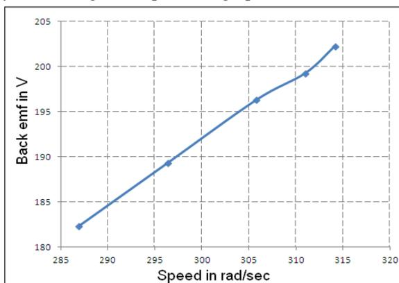
Fig. 3 Variation of speed Vs backemf
