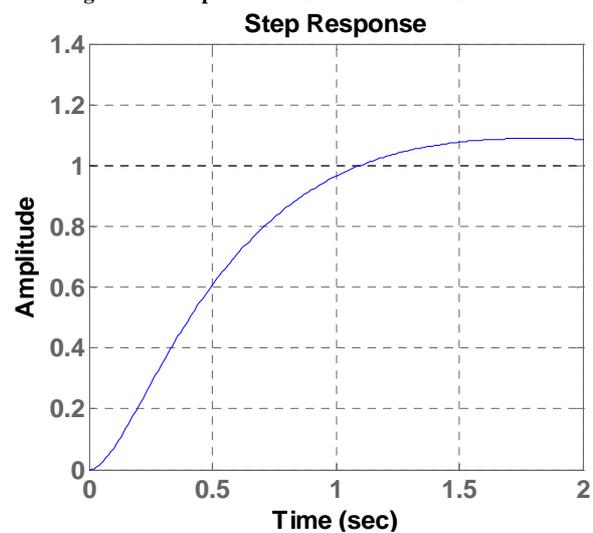
Fig. 10 Time response of DC motor with PI-Controller
