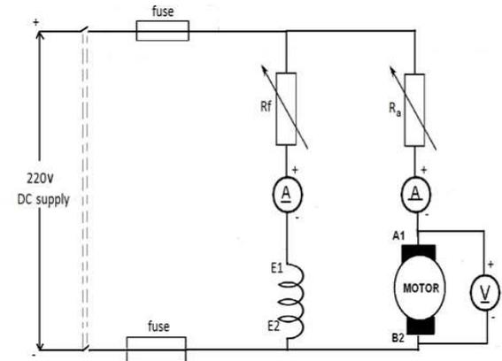
Fig. 2 Experimental circuit for speed control test
