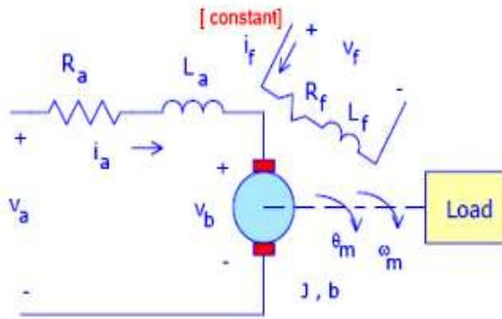
Fig. 1 Mathematical model of DC Motor
