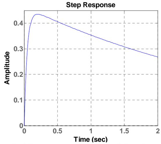
Fig. 8 Time response of DC motor with D-Controller
