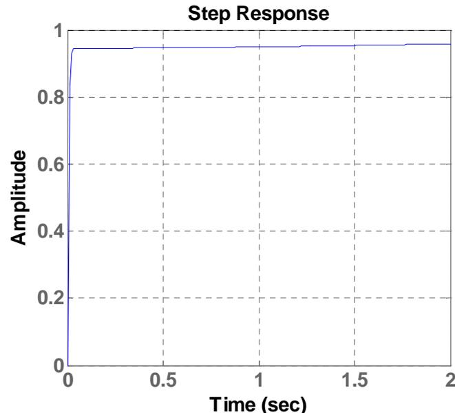
Fig. 13 Time response of DC motor with PID-Controller
