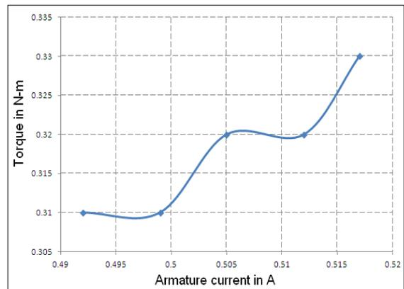
Fig. 4 Variation of armature current Vs Torque
