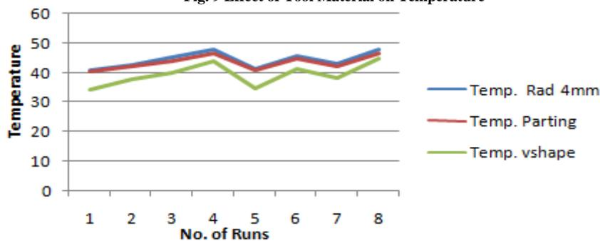
Fig. 10 Effect of Tool Shape on Temperature
