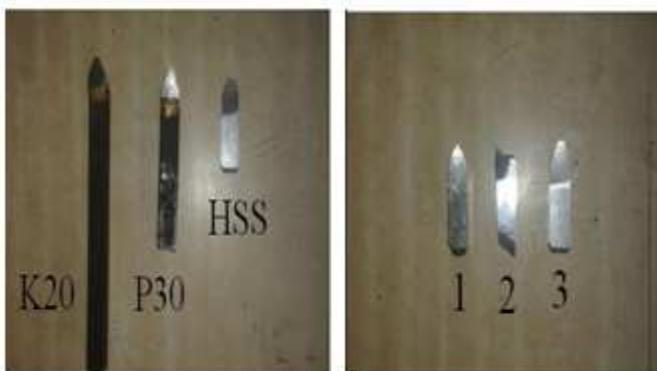
**Fig. 5 Different Tool Materials & Shapes**
