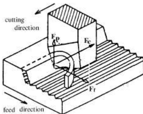
**Fig. 3 Mechanism of Shaping Operation [17]**
