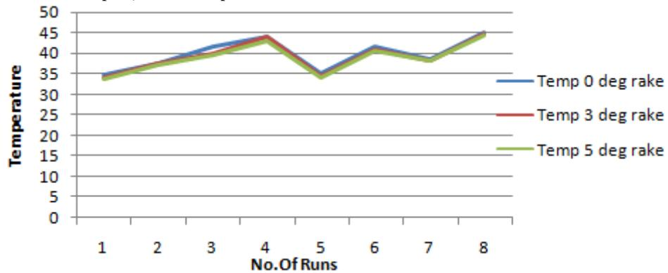
Fig. 8 Effect of Tool Rake on Temperature
