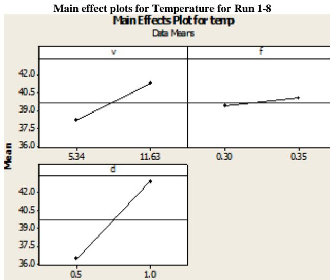
Fig. 6 Temperature Variation V/S Speed, Feed and Depth of Cut
