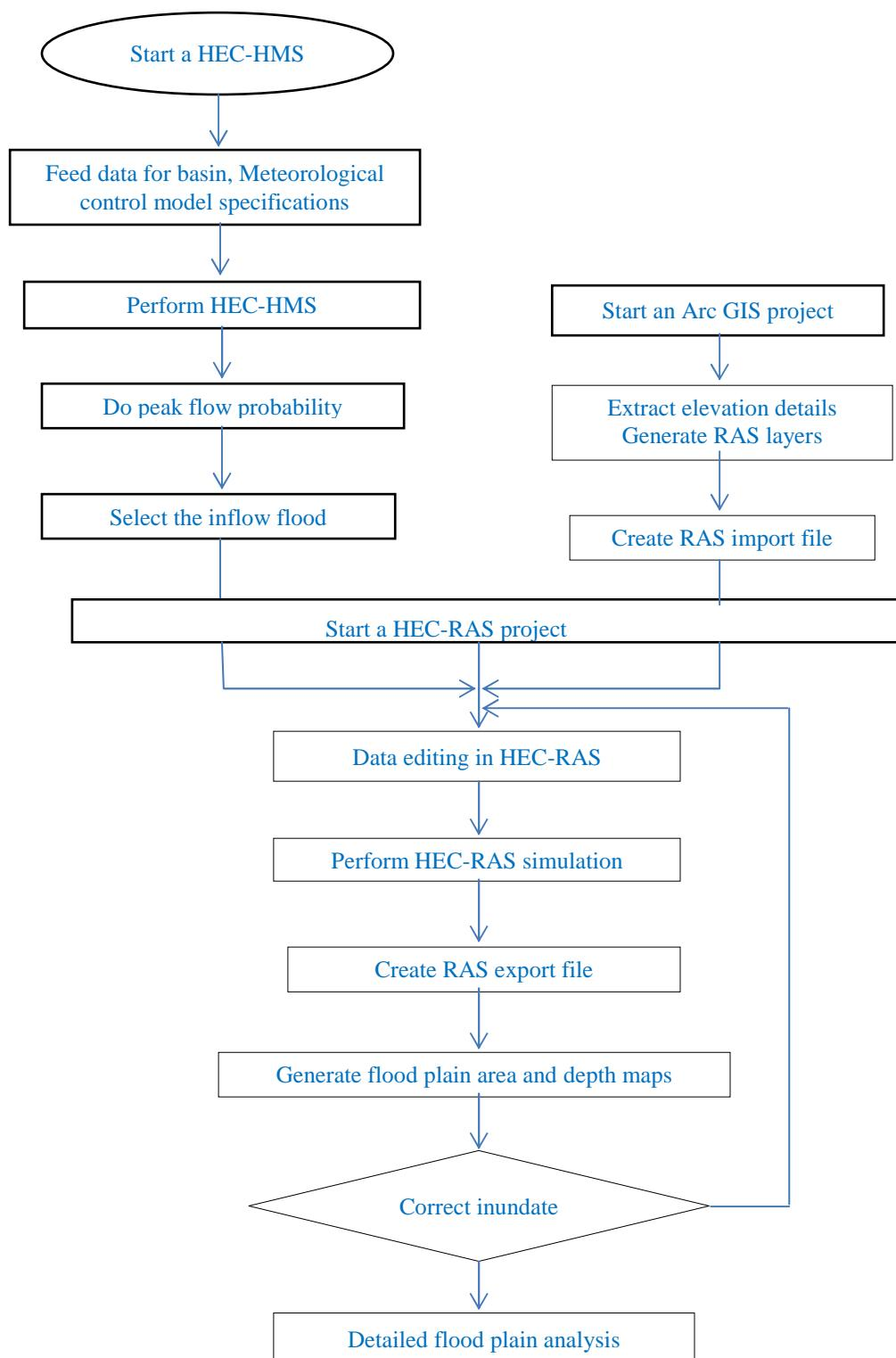
Fig. 1 Methodology flow chart for flood plain modelling
