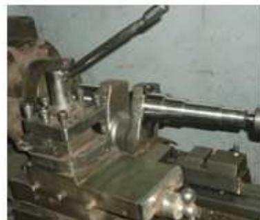
Fig.2 Pin Turning
