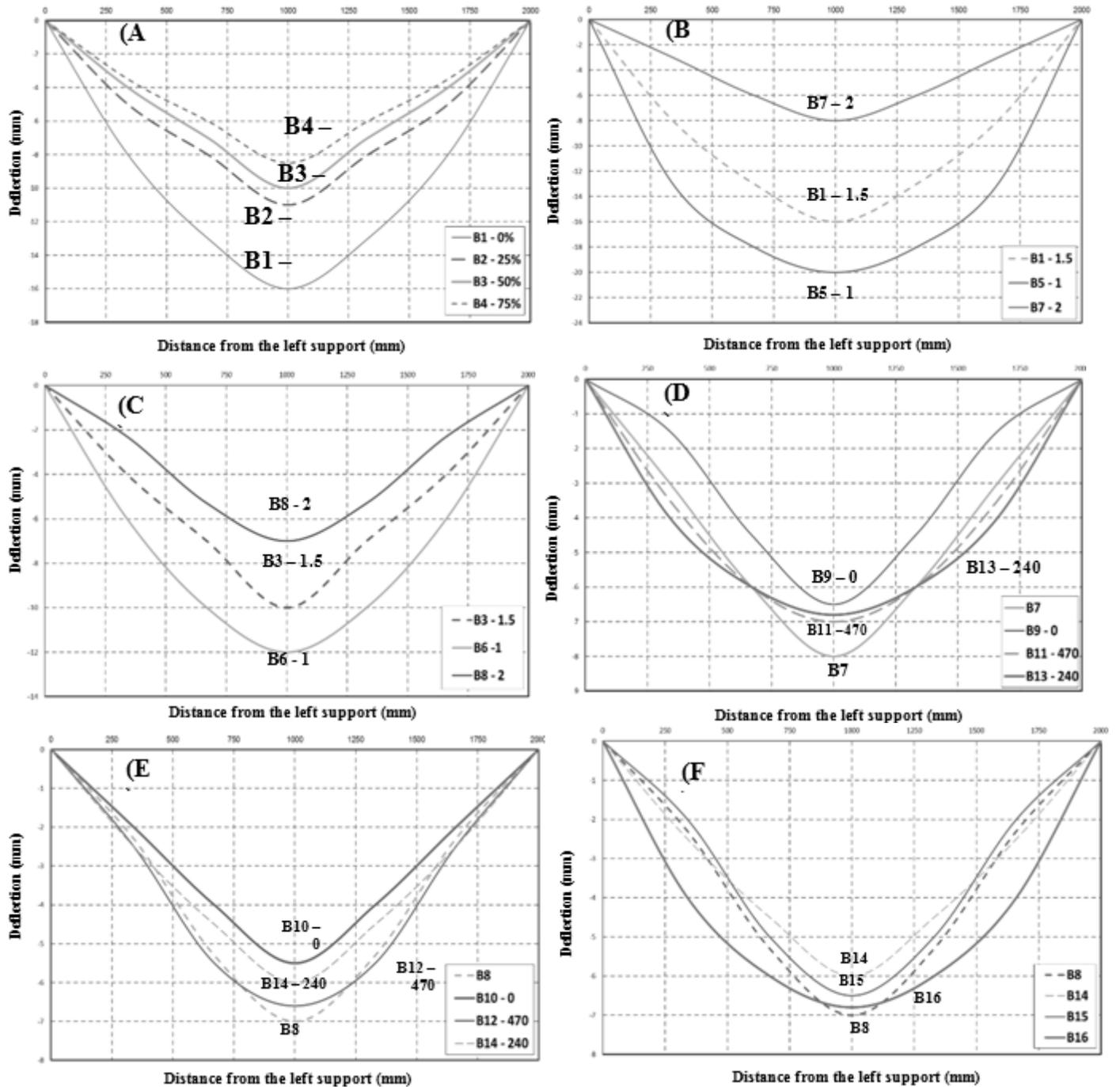
Fig. 7 Deflection Shape at Ultimate Load of the Tested Specimens: (A) Effect of the RCA Ratio, (B) Effect of the Shear Span with 0% Replacement of RCA, (C) Effect of the Shear Span with 50% Replacement of RCA, (D) Effect of the Location of Opening with 0% Replacement of RCA, (E) Effect of the Location of Opening with 50% Replacement of RCA, (F) Effect of the Different Reinforcement Details around Openings
