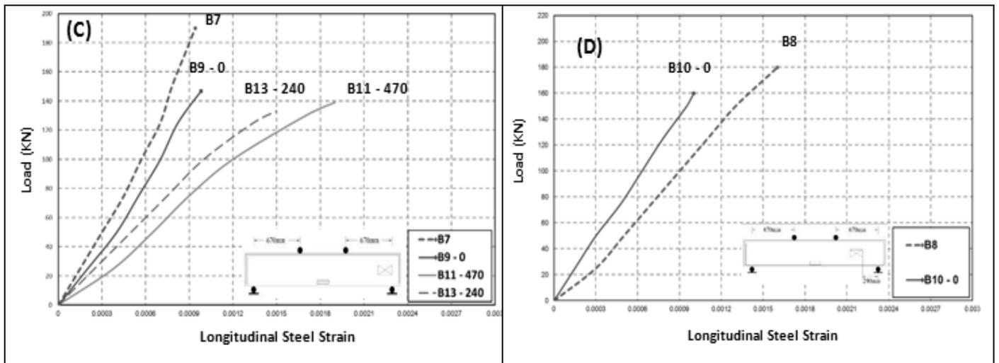
Fig. 9 Load- Longitudinal Steel Strain Relationship of the Tested Specimens: (A) Effect of the Shear Span with 0% Replacement of RCA, (B) Effect of the Shear Span with 50% Replacement of RCA, (C) Effect of the Location of Opening with 0% Replacement of RCA, (D) Effect of the Location of Opening with 50% Replacement of RCA
