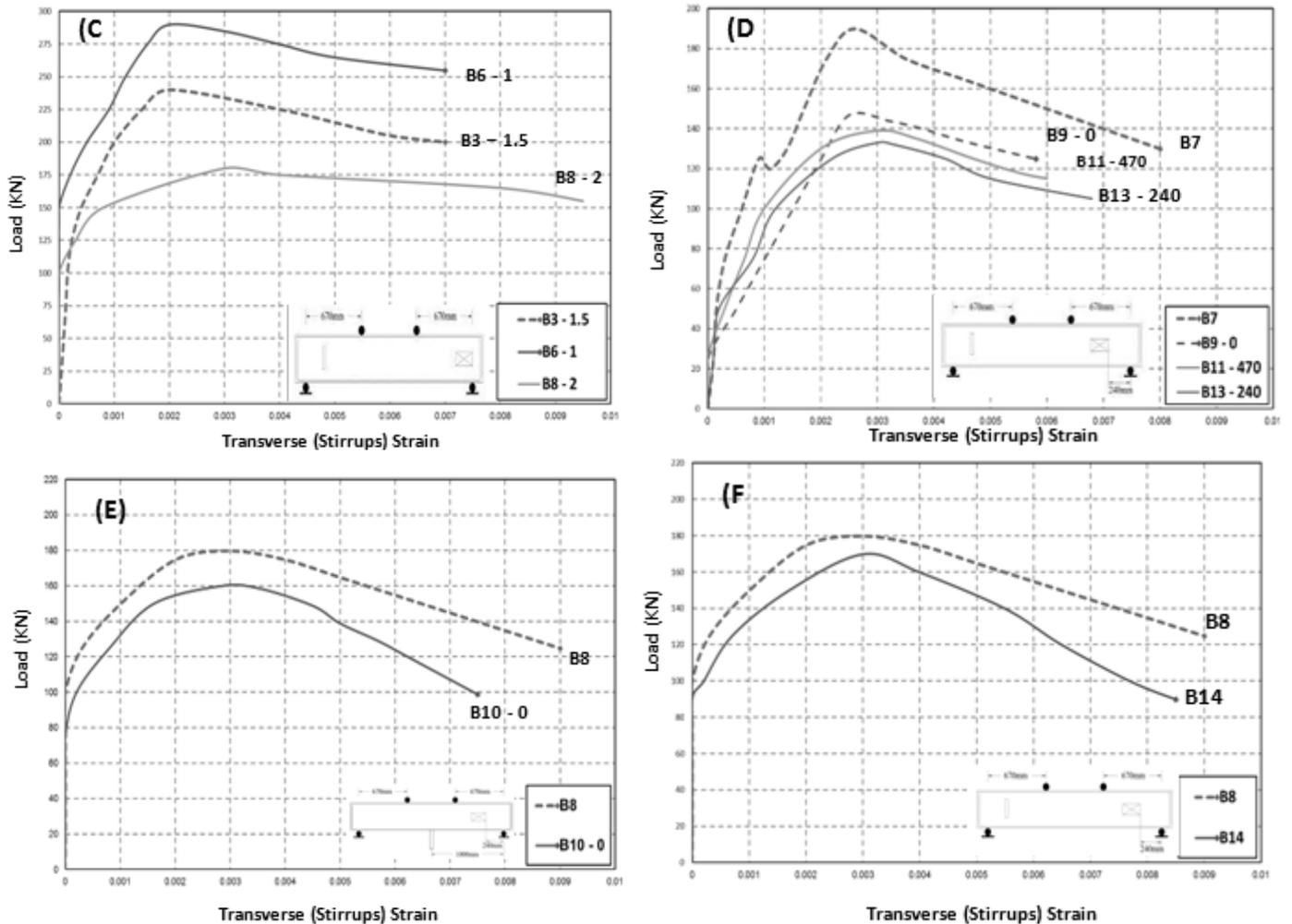
Fig. 8 Load- Transverse Steel Strain Relationship of the Tested Specimens, (A) Effect of the RCA Ratio, (B) Effect of the Shear Span with 0% Replacement of RCA, (C) Effect of the Shear Span with 50% Replacement of RCA, (D) Effect of the Location of Opening with 0% Replacement of RCA, (E) Effect of the Location of Opening with 50% Replacement of RCA, (F) Effect of the Different Reinforcement Details around Openings
