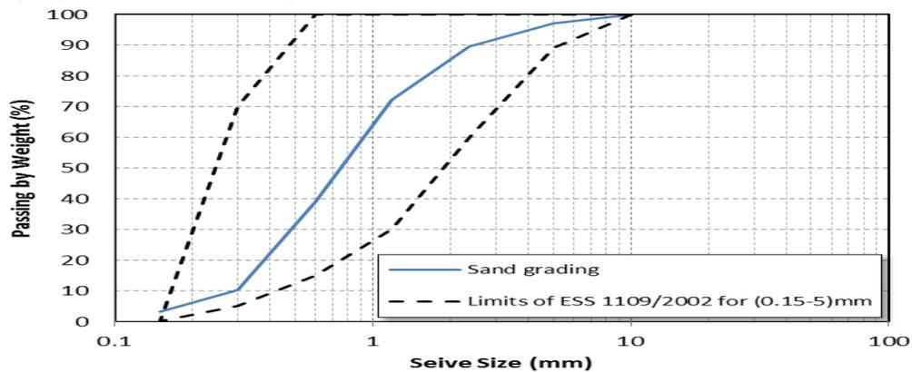
Fig. 1 Grading of Fine Aggregate
