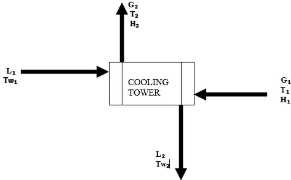
Fig. 2 Scheme of the Energy Balance Calculation
