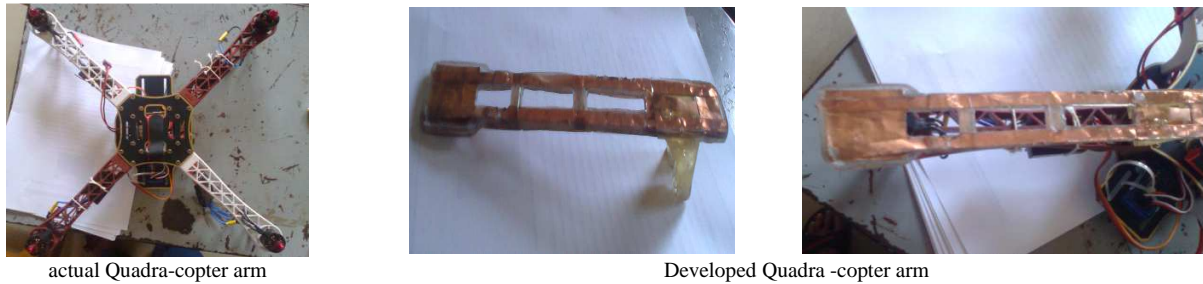
Fig. 4The actual quadra-copter arm and smart material quadra-copter arm
