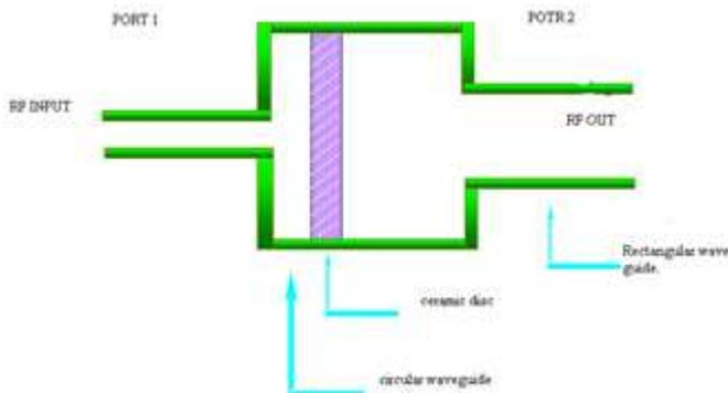
**Fig. 1 Schematic diagram of Asymmetric pillbox type RF window**
