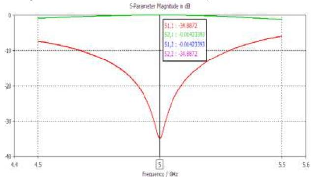
**Fig. 6 Simulated Return loss and Insertion loss of asymmetric window**
