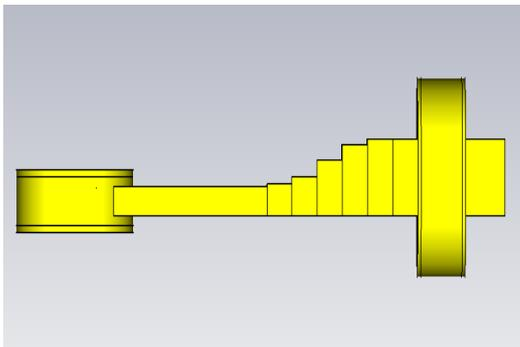
**Fig. 3 RF window with transformer & cavity**
