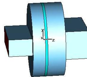
**Fig. 2 3D view of Asymmetric pillbox type RF window**
