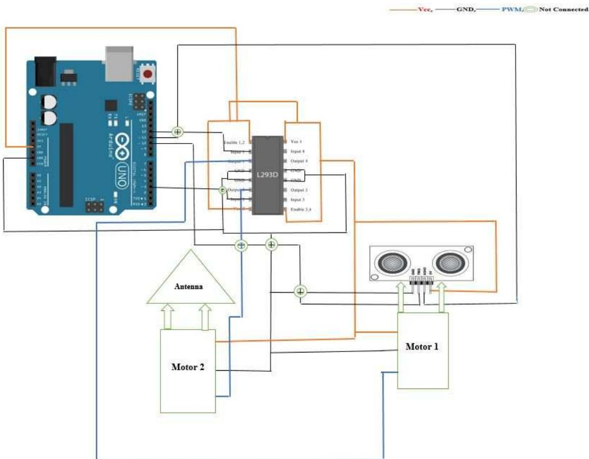
Fig.3 Circuit Diagram of the designed system
