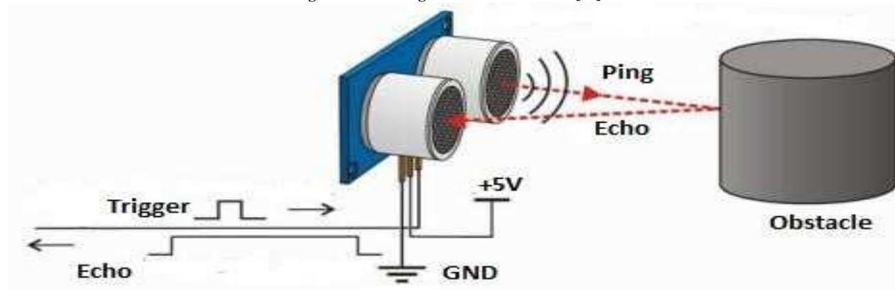
Fig.7 Working of Ultrasonic Sensor [12]
