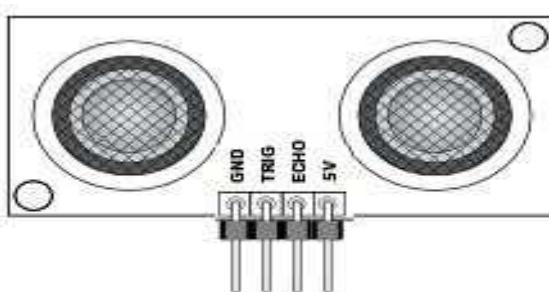
Fig.5 Ultrasonic Sensor [10]
