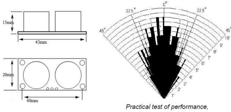
Fig.6 Radiation Angle of Ultrasonic Sensor [11]
