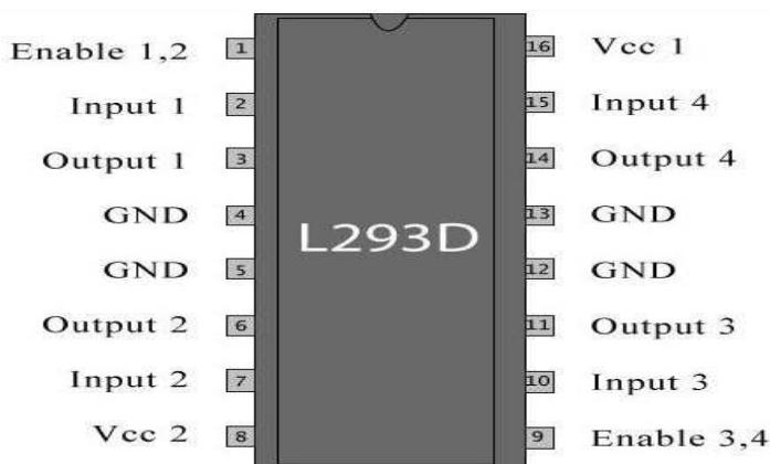
Fig.8 Pin configuration of L293D [13]
