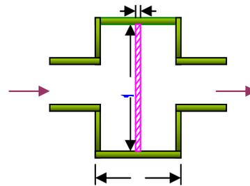
Fig. 1 Schematic view of pillbox type RF window
