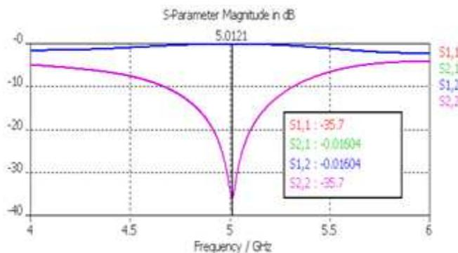
Fig. 2 Plot of Return Loss & Insertion Loss
