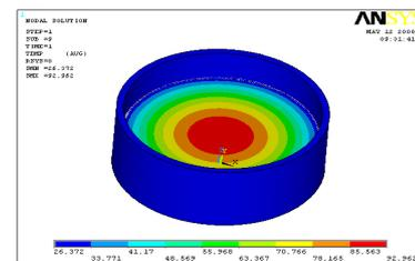
**Fig. 3 Temperature profile for loss 30.95 W**
