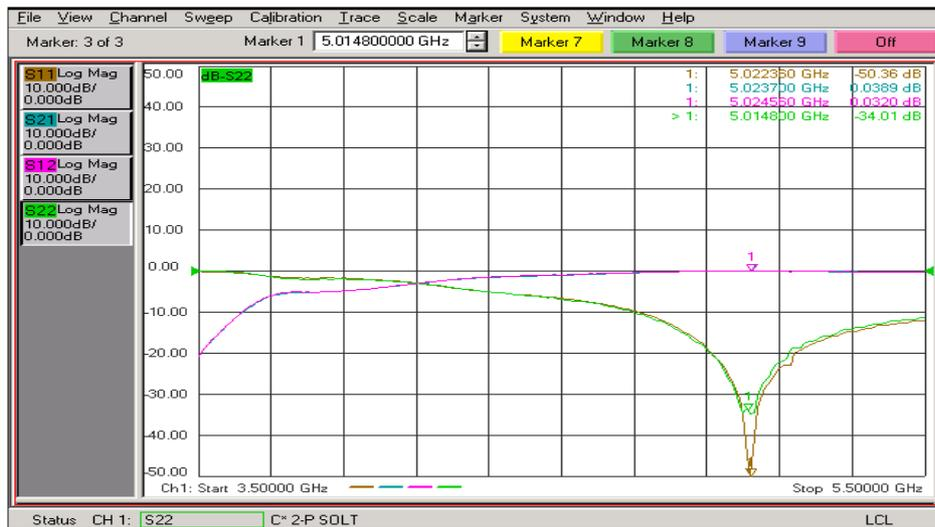
**Fig. 5 Measured Return Loss & Insertion Loss of the window**
