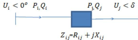
Fig.3 2-Bus Line Model for derivation of Voltage Stability Indices
