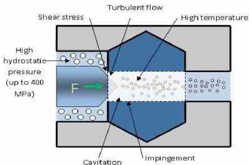
Fig. 7 Various physical phenomena simultaneously affecting a fluid during high pressure homogenization
