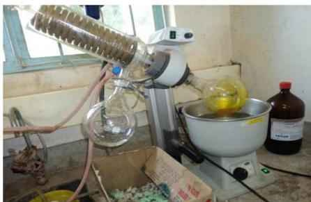
Fig. 3 Rotary Evaporator set for recovering Hexane from Palm Oil
