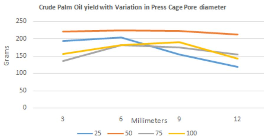
Fig. 16 Crude Palm Oil yield with Variation in Press Cage Pore diameter
