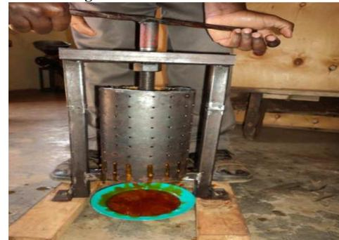
**Fig. 10** Press cage extracting Palm Oil from the mash
