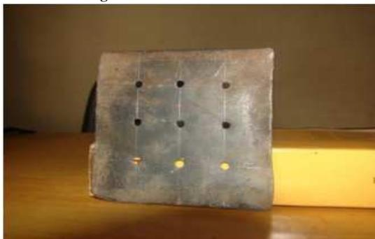
**Fig. 9** The 3 mm diameter holes
