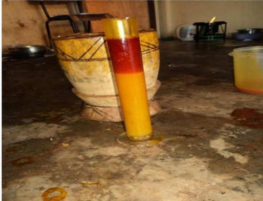
Fig. 13 A column of mechanically extracted oil showing clarified Palm Oil at the top and water soluble impurities at the bottom
