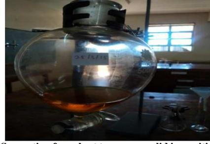
Fig. 4 Separation funnel set to remove solid impurities from clarified Palm Oil
