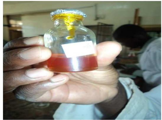
**Fig. 14 A sample of Hexane extracted Palm Oil**
