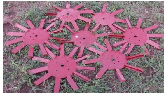
Fig. 1 The Assembled Runners with 6 to 12 V-Blades
