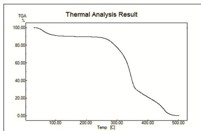
Fig. 4 Thermogram of Raw SR Fibre
