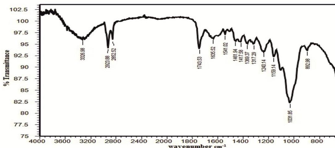
Fig. 2 FTIR spectra of SR Raw Fibre
