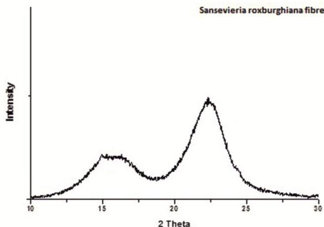
Fig. 3 XRD Diffraction Pattern of SR Fibre
