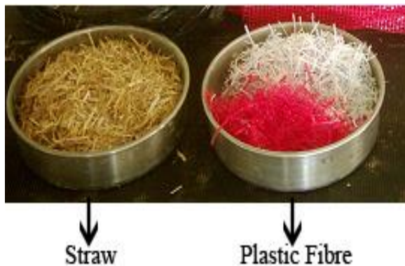
Fig. 3 The fibres used in mud brick production
