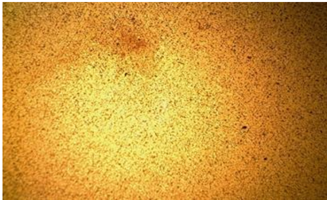
Fig.7 Full martensite structure: Medium carbon steel quenched in agitated water-based eggshells powder quenchant. (X250)
