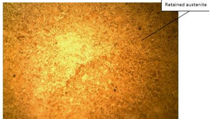
Fig.8 Martensite structure with retained austenite: Medium carbon steel quenched in unagitated water-based eggshells powder quenchant. (X250)
