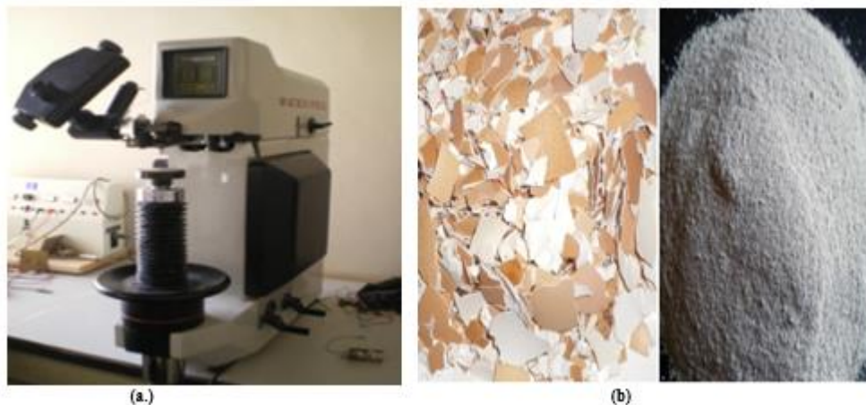
Fig.1 (a) Digital Rockwell Hardness Machine (b) Eggshell before and after grinding Pattern
