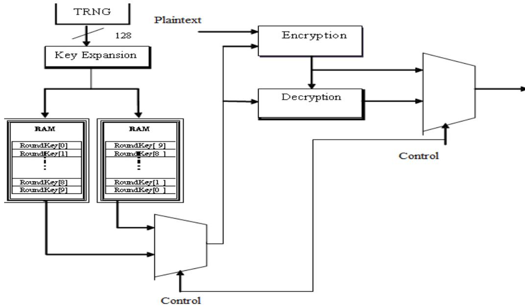
Fig. 12 Architecture for encryption/decryption in single-chip
