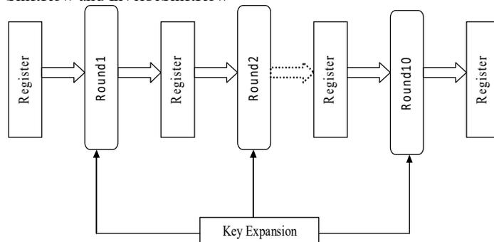
Fig.1 Fully-pipelined AES architecture
