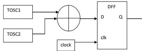
Fig. 4 The structure of proposed TRNG [9]
