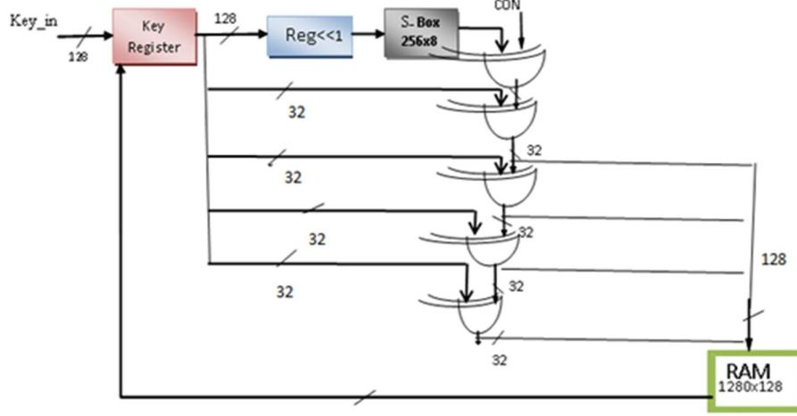
Fig. 11 Architecture for Key Expansion
