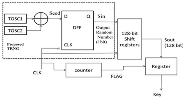
Fig. 5 Architecture for Cryptographic Key Generator
