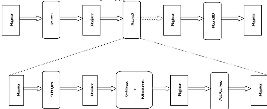
Fig. 2 Sub-pipelined AES
