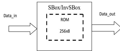
Fig.6 Implementation of SubByte/InvSubByte
