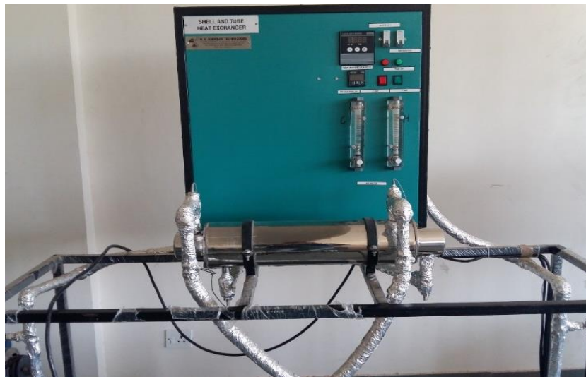
Fig. 1 Experimental Set-up of shell and tube heat exchanger
