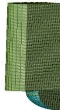
Fig.1 Computational grid with boundary surfaces at TDC at 720° CA Fig.2 Computational grid with boundary surfaces at BDC at 800° CA
