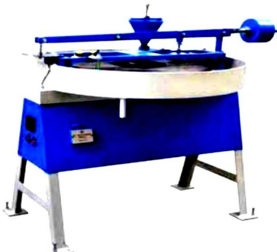
Fig. 1 Abrasion resistance testing machine
