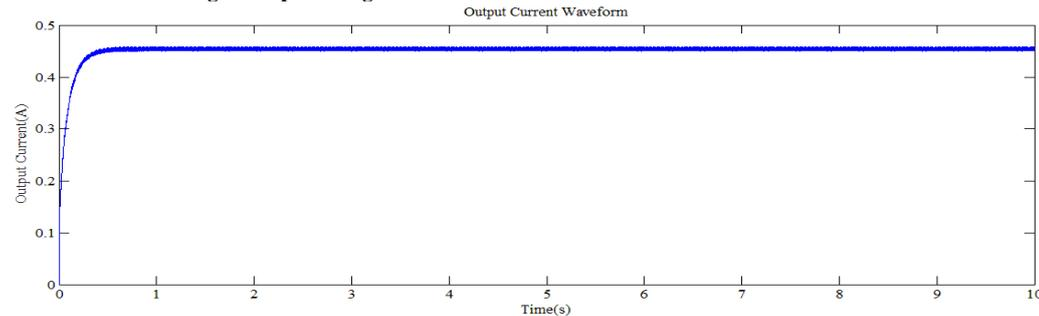
**Fig. 7 Output current waveform of ordinary SEPIC converter**
