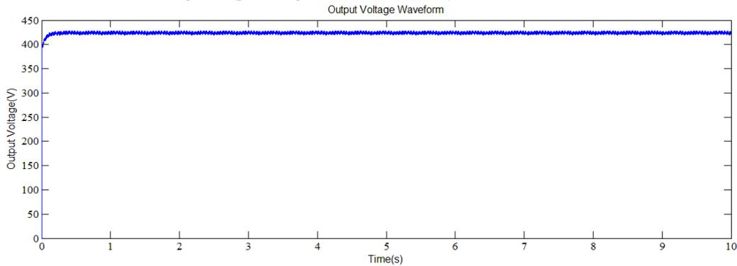
**Fig. 6 Output voltage waveform of SEPIC converter with snubber circuit**
