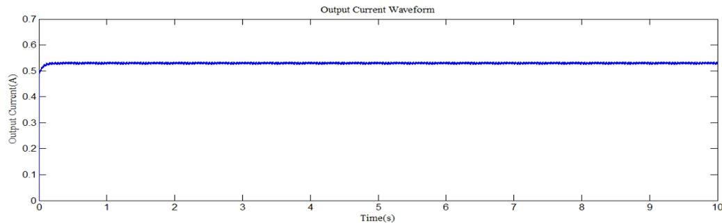
Fig. 8 Output current waveform of SEPIC converter with snubber circuit
