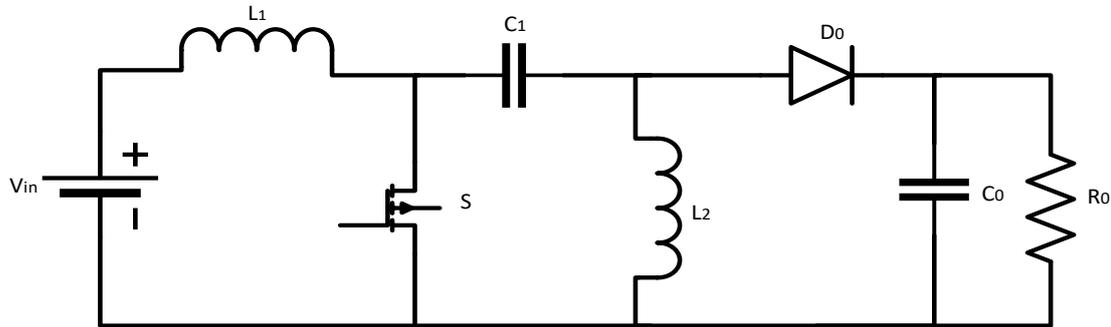
Fig. 1 Circuit diagram of SEPIC converter
