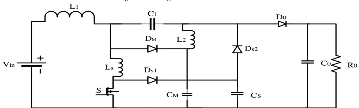
Fig. 2 Circuit diagram of SEPIC converter with Snubber Circuit
