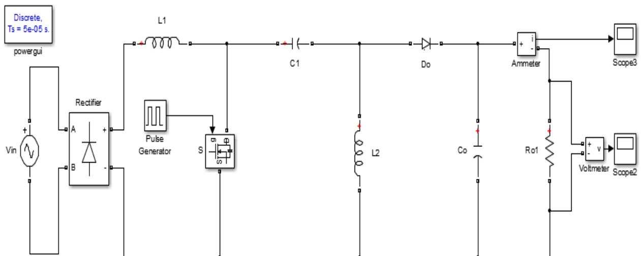
Fig. 3 Simulink model for ordinary SEPIC converter
