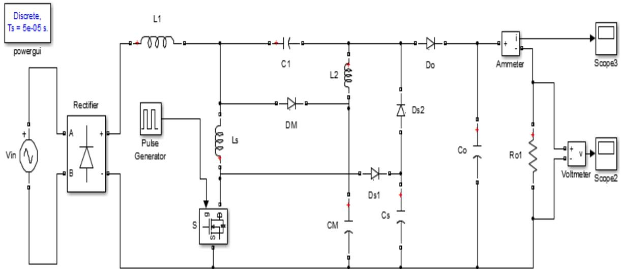
**Fig. 4 Simulink model for SEPIC converter with snubber circuit**
