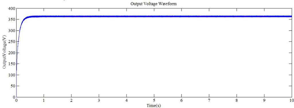
**Fig. 5 Output voltage waveform of ordinary SEPIC converter**
