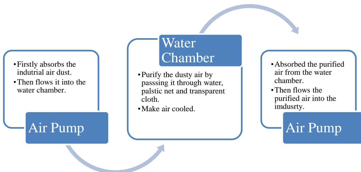
**Fig. 1** Flow chart of working principles for Industrial Air Dust Removing and Air Cooling Machine
