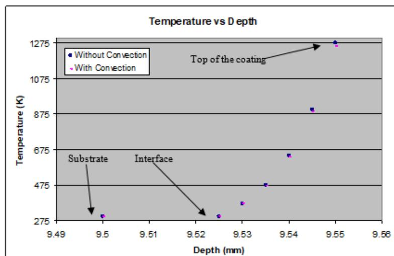
**Fig. 11** Temperature profile for transient analysis of the coating region (from the top of the coating to just below the interface in figure 7) at  $t = 0.0039$  s (boundary conditions equations 20, 21, 22 and initial condition equation 23)
