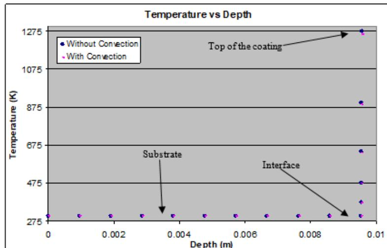
**Fig. 10** Temperature profile for transient analysis at  $t = 0.0039$  s (boundary conditions equations 20, 21, 22 and initial condition equation 23)
