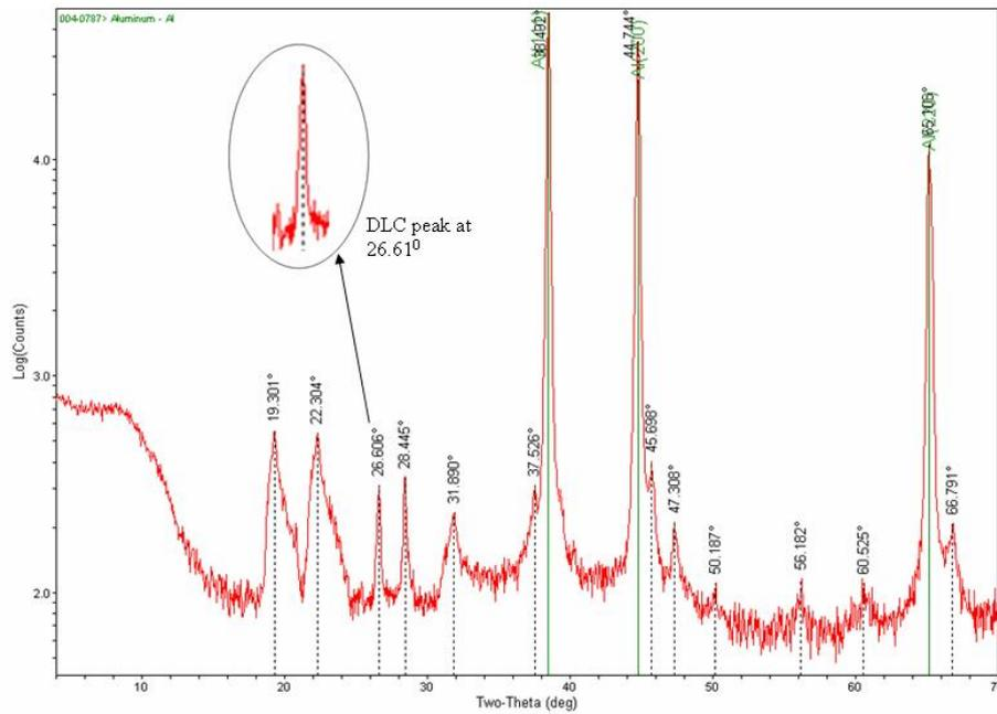
Fig. 5 XRD diffraction pattern of laser-sintered sample using copper  $K_{\alpha}$  radiation
