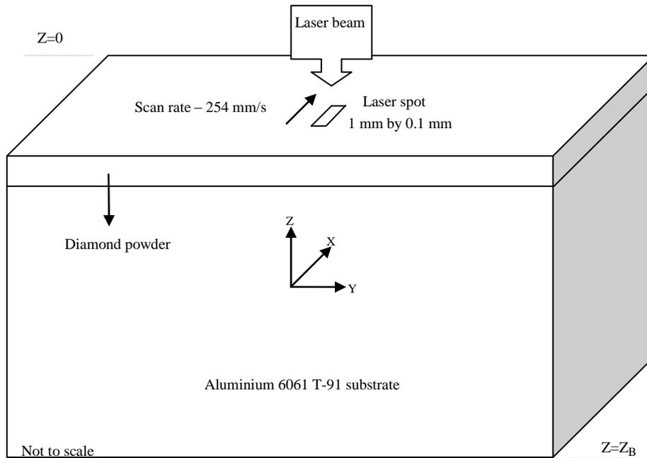
**Fig. 3** Three-dimensional representation of the thermal model
