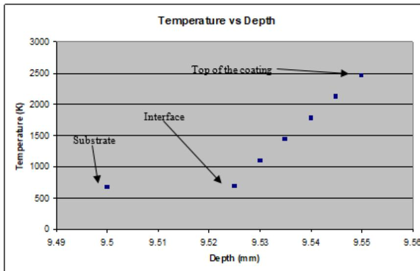
Fig. 8 Temperature profile for the steady state analysis for the coating region (from the top of the coating to just below the interface in figure 4) (boundary conditions equations 17, 18 and initial condition equation 23)
