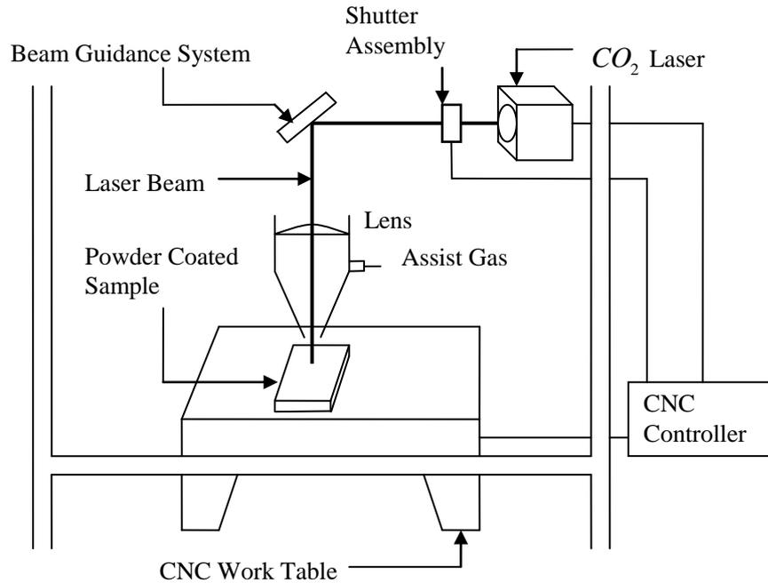
**Fig. 1** Schematic diagram of the direct laser-sintering process
