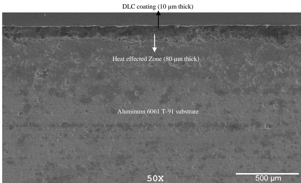
**Fig. 2** SEM micrograph of the transverse section of the coating
