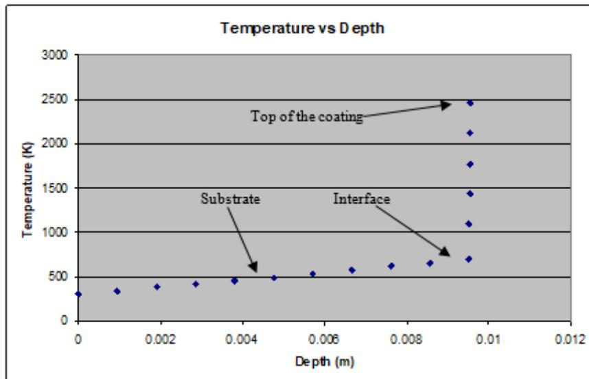
Fig. 7 Temperature profile for one-dimensional steady state analysis (boundary conditions equations 17, 18 and initial condition equation 23)
