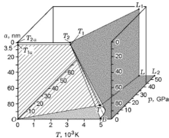
**Fig. 9** Phase diagram of ultrafine carbon [37]:  $OBTT_1T_{1a}$  is the existence domain of the graphite phase,  $OTT_1T_{1a}$  is the interface between the graphite and diamond phases,  $BTT_1$  is the interface between the liquid carbon and graphite phases, and  $TT_2L_1L$  is the interface between the liquid carbon and diamond phases
