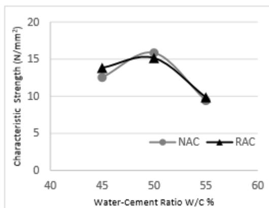
**Fig. 3.3** Characteristic strength (MPa) at 7days
