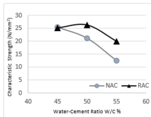
**Fig. 3.4** Characteristic strength (MPa) at 28days
