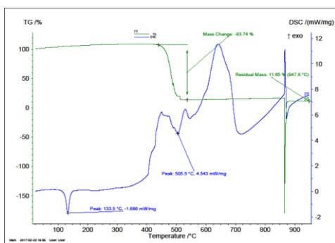
Fig. 6 TGA & DSC curve of HDPE
