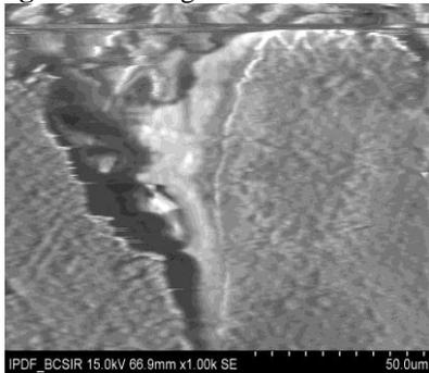
**Fig. 11** SEM image of untreated BNHF-HDPE composite
