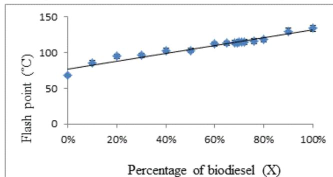
Fig. 3 Measured flash points versus percentage of biodiesel
