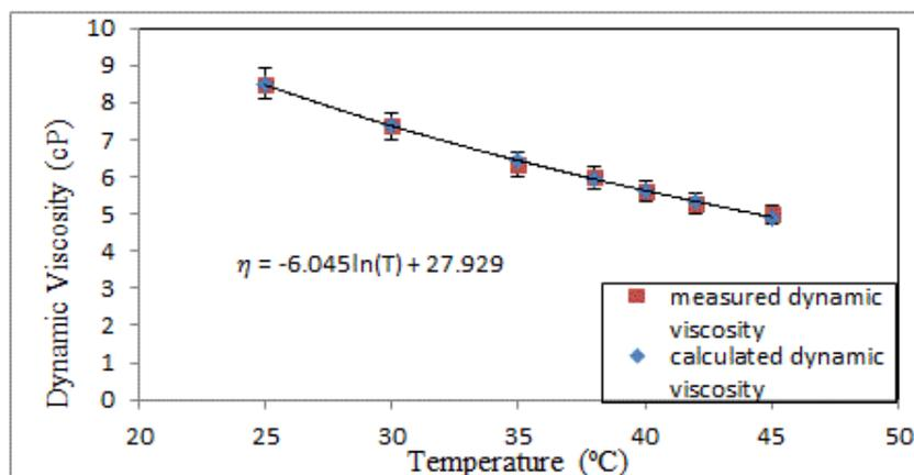
Fig. 7 Measured and calculated values of dynamic viscosity as a function of temperature of B100 sample from Eq. (12)
