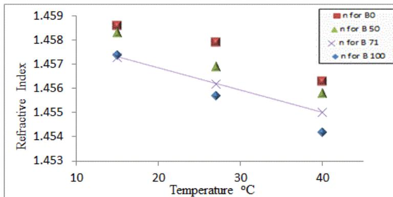
Fig. 2 Measured Density refractive indices versus temperature for B100, B71, B50, and B10
