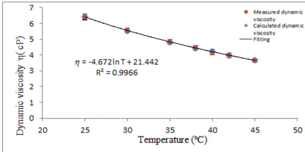
Fig. 6 Measured and calculated values of dynamic viscosity as a function of temperature of B71 sample from Eq. (12)
