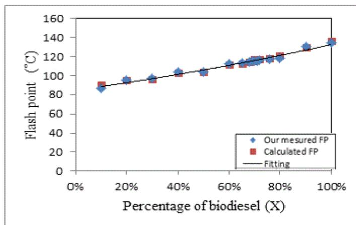
**Fig. 4** Measured and calculated values of flash points using exponential formula Eq. (10)
