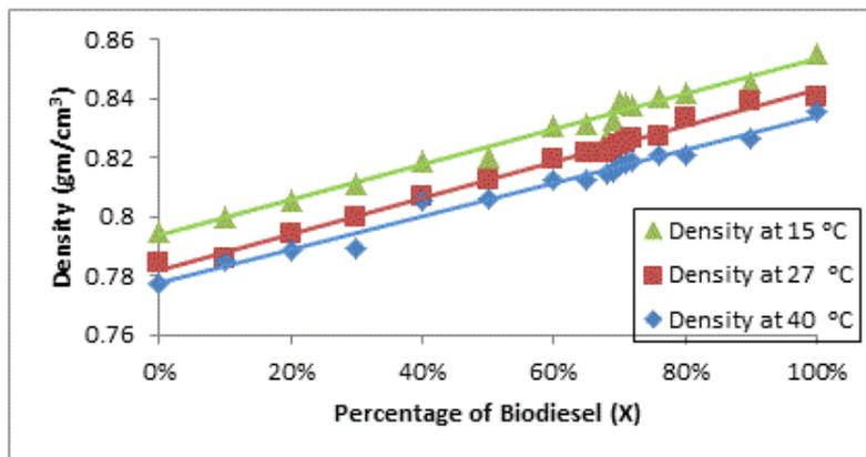
Fig. 1 Density versus percentage of biodiesel at 15 °C, 27 °C, and 40 °C
