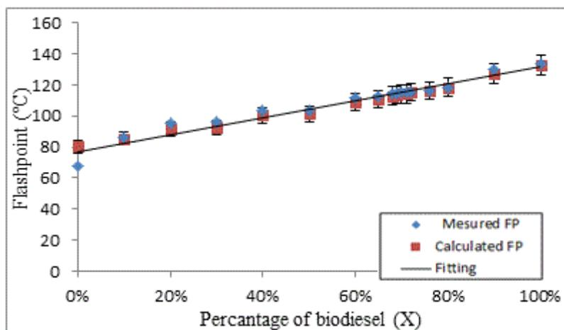
**Fig. 5** Measured and calculated values of flash points using linear formula Eq. (11)
