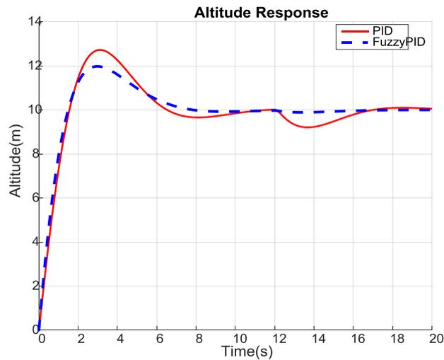
**Fig. 7** Altitude response for PID and FuzzyPID control
