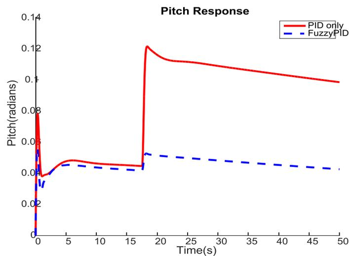
Fig. 5 Pitch response for PID and FuzzyPID control
