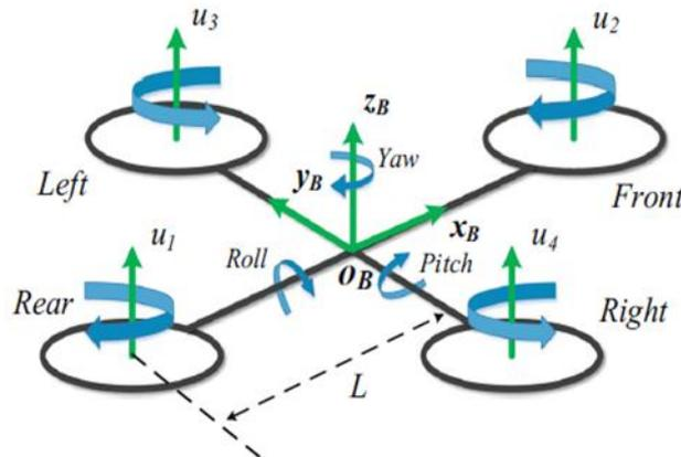
Fig. 1 Schematic representation of a Quadrotor UAV system
