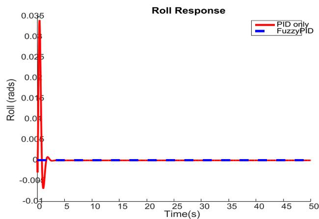
Fig. 6 Roll response for PID and FuzzyPID control
