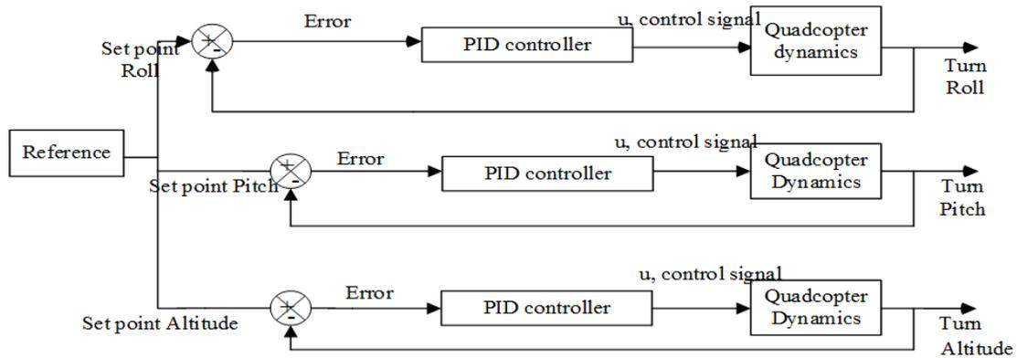
Fig. 2 PID control block diagram
